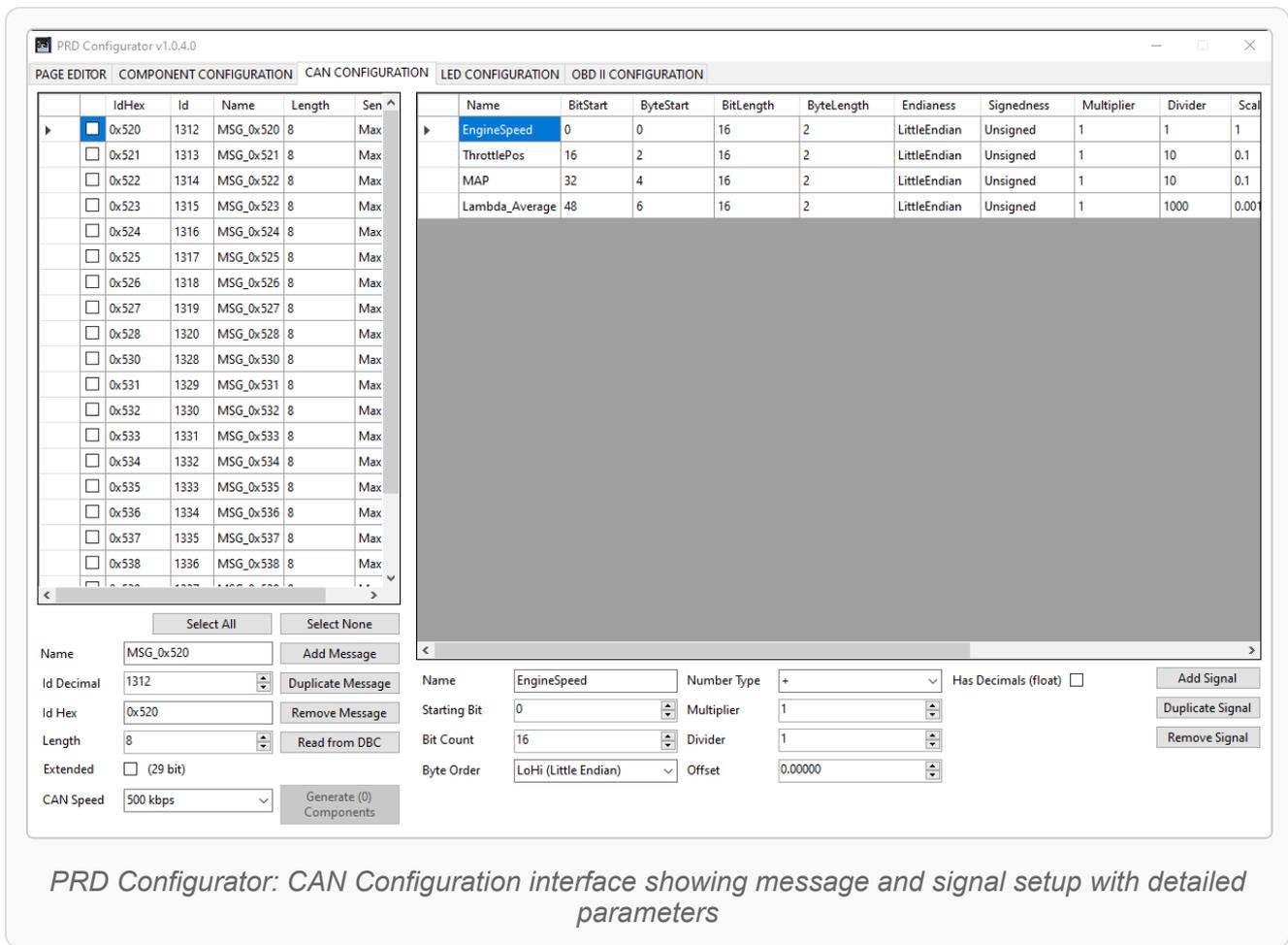
*PRD Configurator: CAN Configuration interface showing message and signal setup with detailed parameters*
