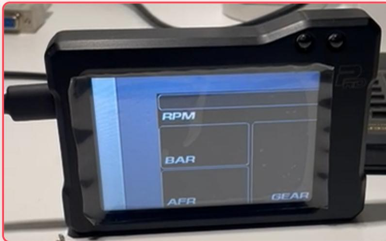
**⚠ Problem Example:** Interface distortion when Windows scaling is not set to 100%
