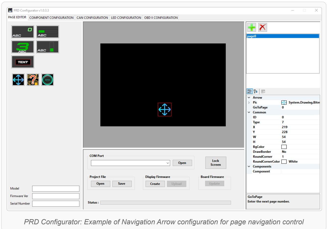
PRD Configurator: Example of Navigation Arrow configuration for page navigation control
