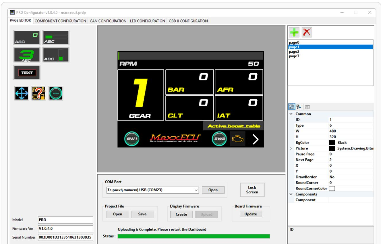
PRD Configurator: Example of a complete racing dashboard showing RPM gauge, gear indicator, engine parameters (BAR, AFR, CLT, IAT), control buttons, and navigation
